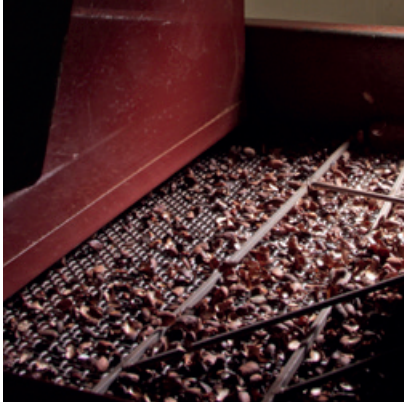
SEPARATION OF COCOA SHELLS FROM COCOA NIBS
