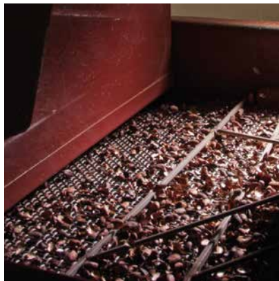
SEPARATION OF COCOA SHELLS FROM COCOA NIBS
