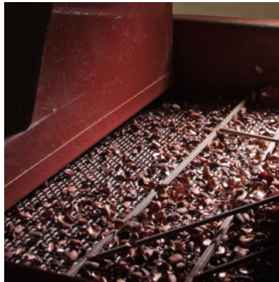
SEPARATION OF COCOA SHELLS FROM COCOA NIBS
