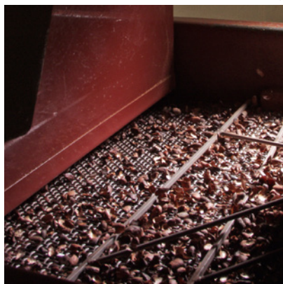
SEPARATION OF COCOA SHELLS FROM COCOA NIBS
